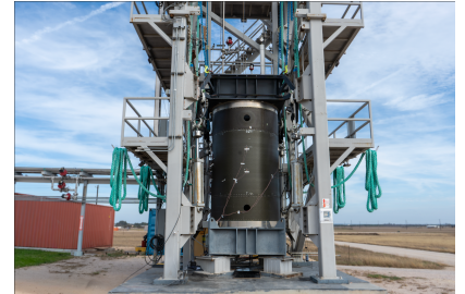
Qualification testing underway for Alpha Block II second stage hardware for Flight 8 on Firefly's test stand at its Rocket Ranch in Briggs, Texas.
