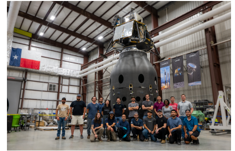
Firefly's Blue Ghost Mission 2 structure qualification model fully stacked with Blue Ghost lander, Elytra Dark vehicle, and dual payload attached fitting at Firefly's Rocket Ranch in October 2025
